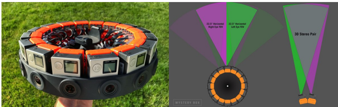
Figure 8. GoPro Odyssey multi camera rig and diagram illustrating a section of the image from each lens generating a stereoscopic image. Image credit: Mystery Box, 2017, https://www.mysterybox.us/blog/2017/1/31/shooting-360-vr-with-gopro-odyssey-and-google-jump-vr .
